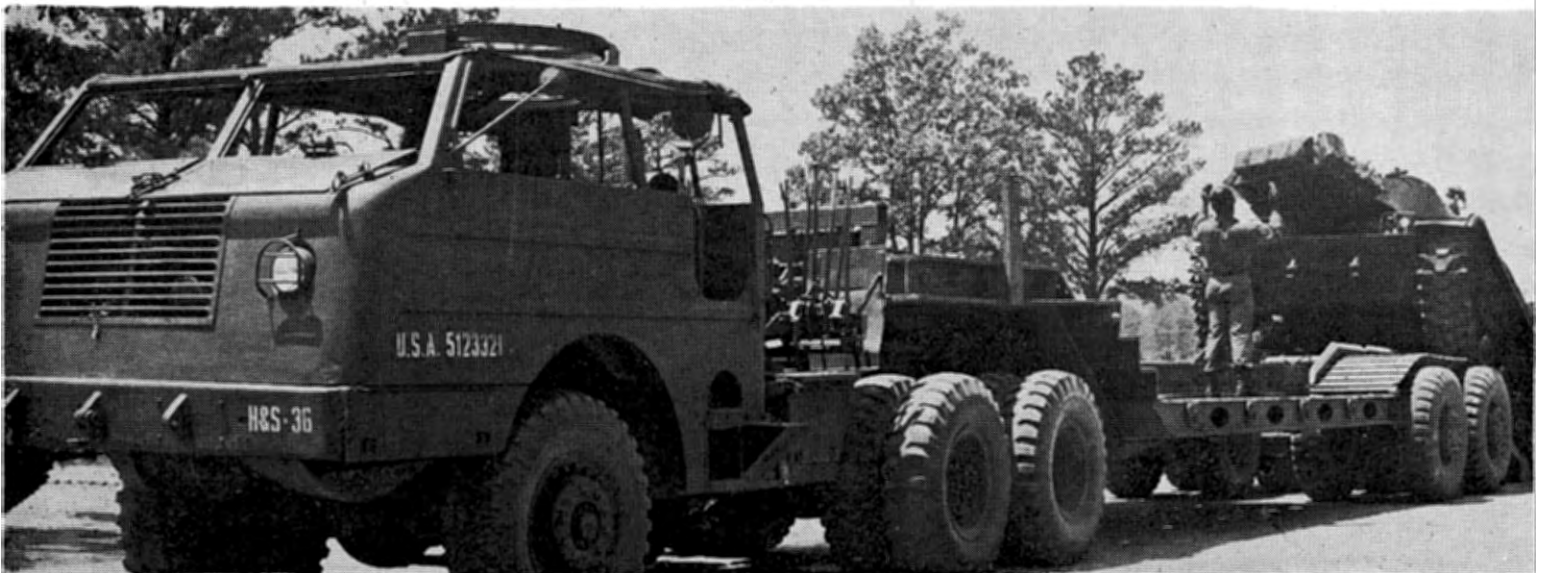
SGT. ROBERT SMITH DIRECTS A T-41 TANK ONTO BATTALION MAINTENANCE'S TANK TRANSPORTER (LOW BOY). THIS MULTI-WHEELED VEHICLE IS USED IN CONJUNCTION WITH THE TANK RECOVERY VEHICLE TO EVACUATE TANKS KNOCKED OUT IN BATTLE.
