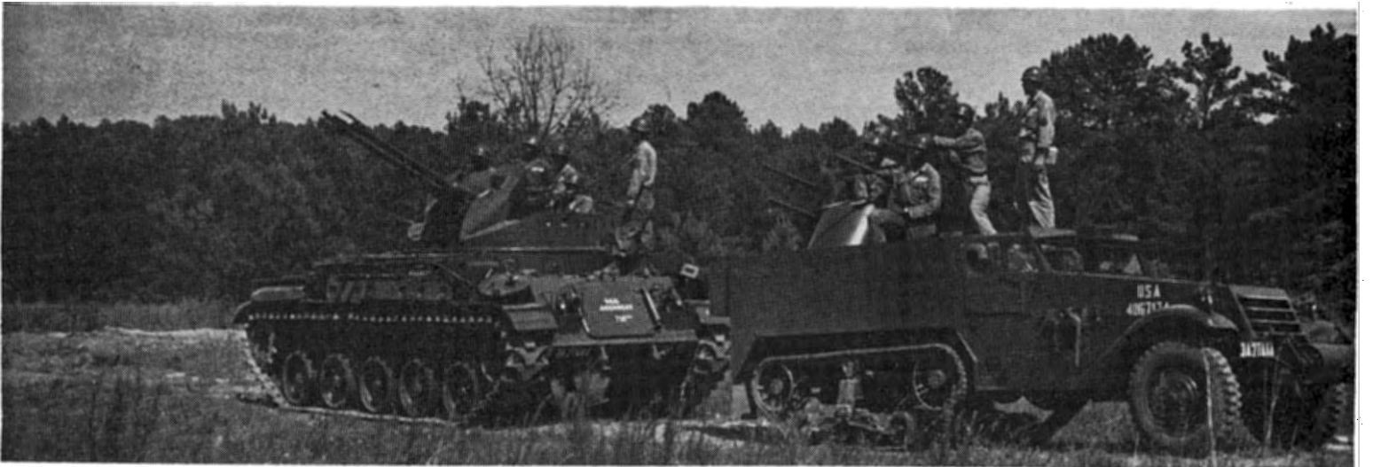
THE 27TH AAA BATTERY IS EQUIPPED WITH THE M-42, MOUNTING THE TWIN 40MM CANNONS, AND THE M-16, MOUNTING THE QUADRUPLE 50 CAL. MACHINE GUNS.
