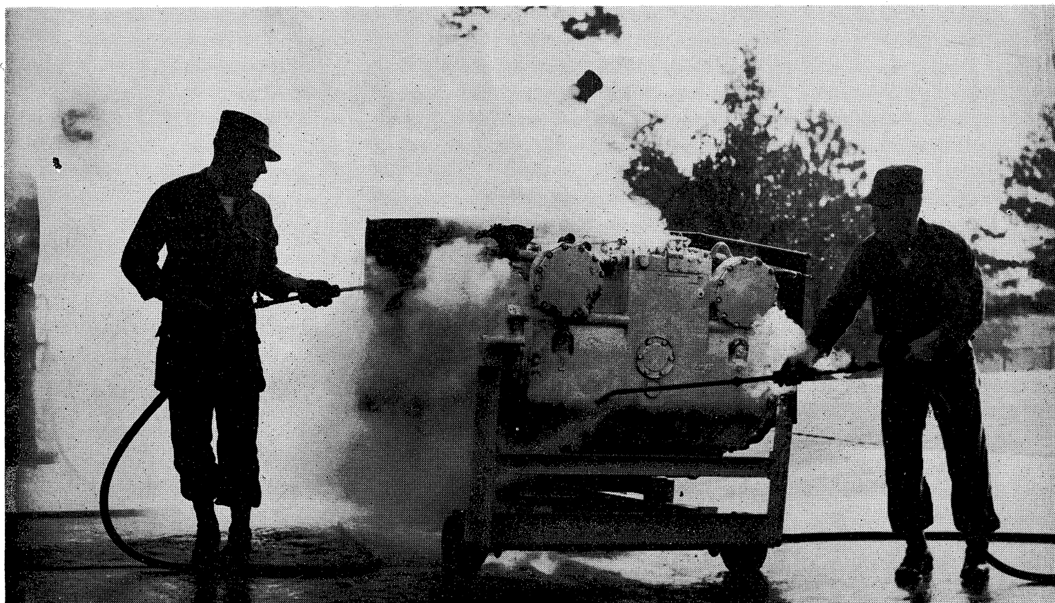
A HUGE M-47 TANK TRANSMISSION GETS A BATH IN STEAM BY TWO MEN FROM HQ. AND SVC. CO. 773D TANK BN, SGT. JOSEPH DALE AND CPL. CECIL JONES.
