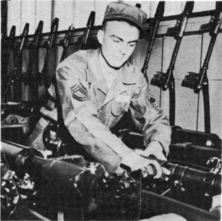
SFC. CLARENCE DURFEE OF WESTERLY, R. I., CHECKS THE TRIGGER MECHANISM OF A 57MM RECOILLESS RIFLE BEFORE IT IS ISSUED TO THE INFANTRY SCHOOL WEAPONS DEPARTMENT FOR CLASSROOM AND DEMONSTRATION PURPOSES. DURFEE IS ONE OF A CREW OF 36 WEAPONS MECHANICS WHO SERVICE THE 50,000 PIECES OF EQUIPMENT ISSUED MONTHLY BY THE HARMONY CHURCH WEAPONS POOL.
