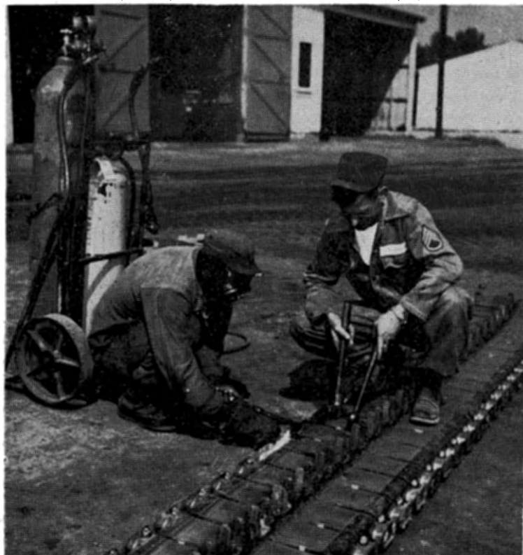
PVT. ROBERT WEST, HQ. AND SVC. CO, 773D TANK BN., AND SGT. JOSEPH J. MARYEK, CO. A, 773D, BURN OFF WEDGE NUTS ON TANK TRACKS PRIOR TO INSTALLING NEW ONES.
