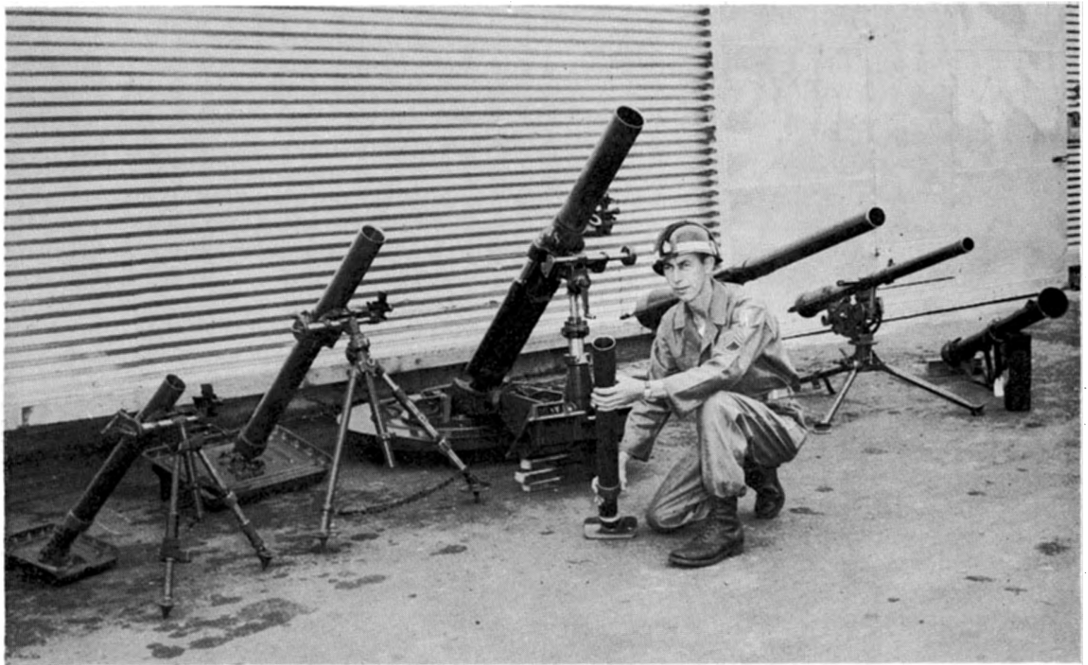
The heavy-weights of the Infantry firepower, officially referred to as crew-seven weapons, are, left to right, the 60 mm mortar, the 81 mm mortar, the 4.2 mortar, the 75 mm recoilless rifle, the 57 mm rifle and the 3.5 rocket launcher. SFC Wallace W. Fleming of Hattiesburg, Miss., holds the 60 mm mortar with hand firing attachment.
