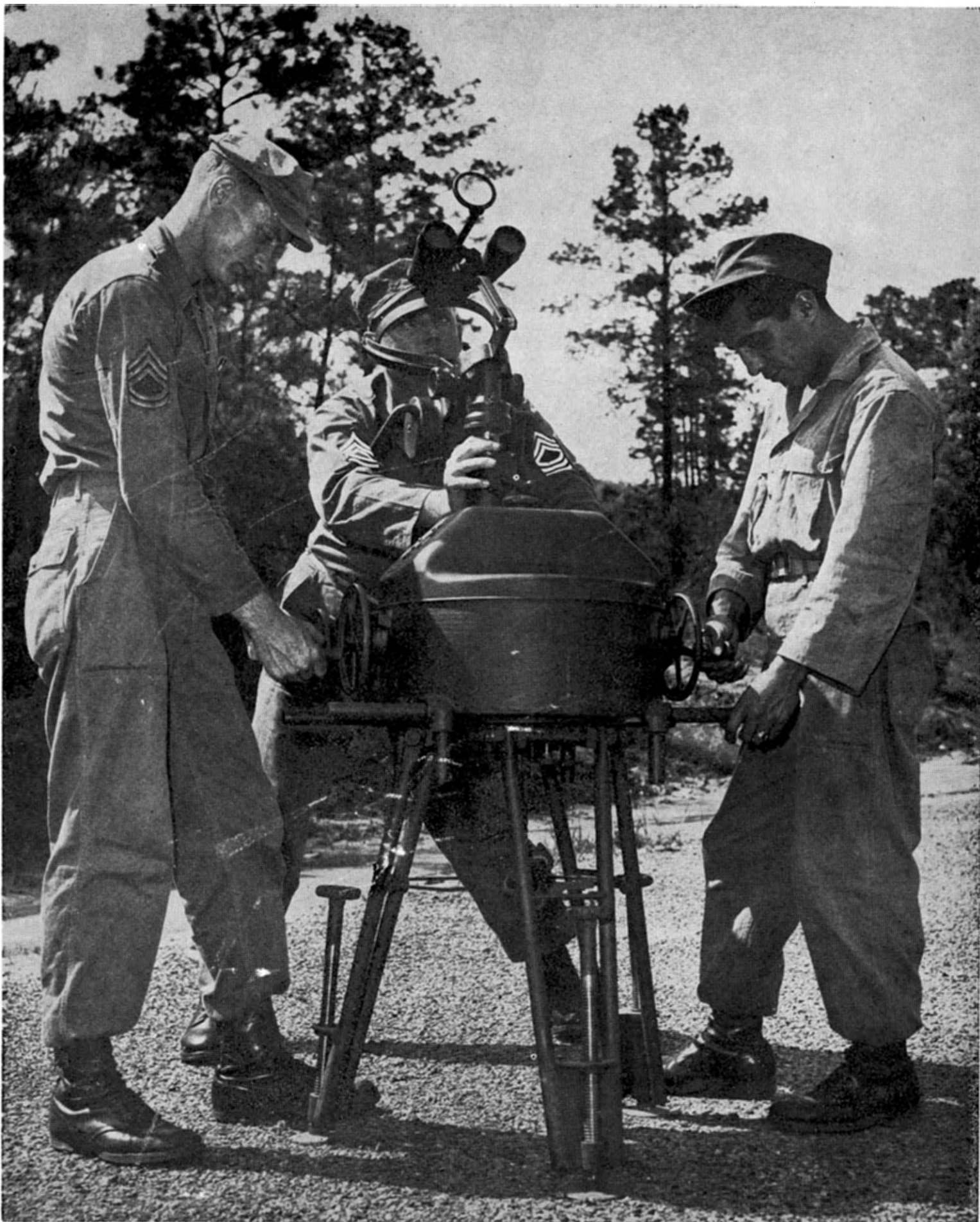
SEARCHLIGHT UNITS EMPLOY A DEVICE KNOWN AS A CONTROL STATION, WHICH AUTOMATICALLY MOVES THESE POWERFUL LIGHTS IN SECONDS. IN THIS PICTURE M/SGT. REX RHODES SIGHTS A PROBABLE TARGET FOR ILLUMINATION. HE IS ASSISTED BY SFC. ARCHIE L. MCKEE AND PVT. JOSEPH VELOZ.
